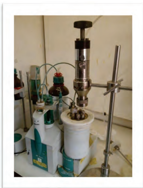
Example of how the Sample Cylinder is used at a the lab under the hood in a refinery
