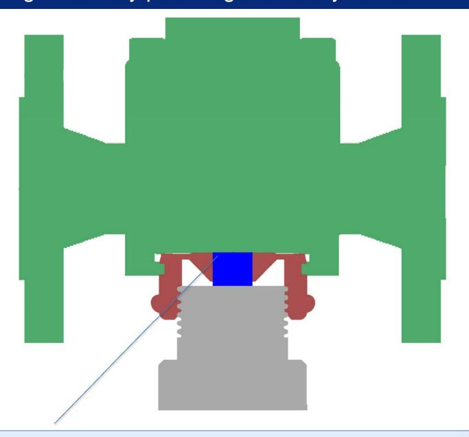
According to the Code of Federal Regulations, "Each open-ended valve shall be equipped with a plug". Our safety plugs have, as standard, a PTFE part - as shown in blue - that acts as secondary containment. By screwing the safety plug tightly into the thread adapter, the outlet of the valve is completely blocked and secondary containment is thus provided. As a result, our valves comply with the Code of Federal Regulations.
