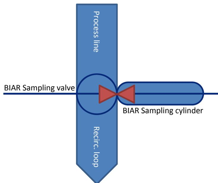
Illustration of the proposed sample method showing the Sample Valve and Sample Cylinder.
