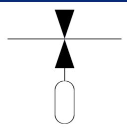
Our sample valves are a specific kind of valve and no standard P&ID symbol can be used to represent it.
