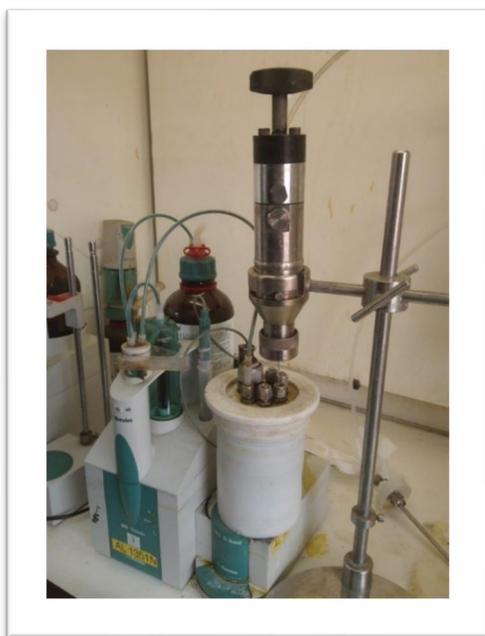
Example of how the Sample Cylinder is used at a the lab under the safety hood in a laboratory
